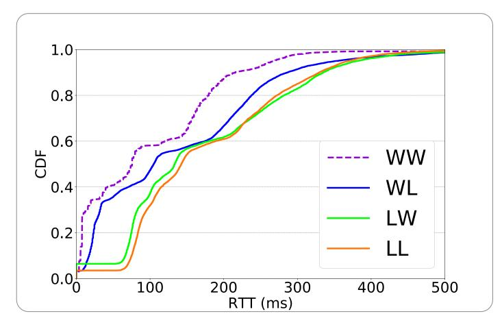
WW: Ping through Wi-Fi interface using address resolved on Wi-Fi DNSWL: Ping through Wi-Fi interface using address resolved on LTE DNSLW: Ping through LTE interface using address resolved on Wi-Fi DNSLL: Ping through LTE interface using address resolved on LTE DNS
